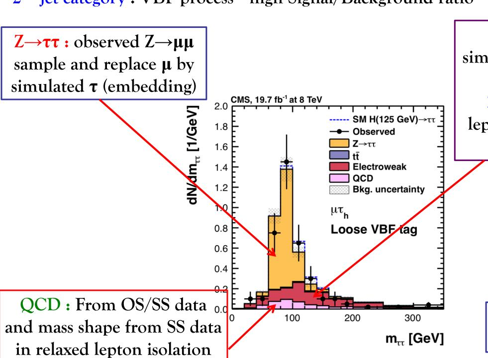
W + jets : Shape from simulation, normalization from  $m_T/P_c$  sideband Z + jets : OS/SS ratio and lepton/jet $\rightarrow \tau$  fakes with shape from simulation
