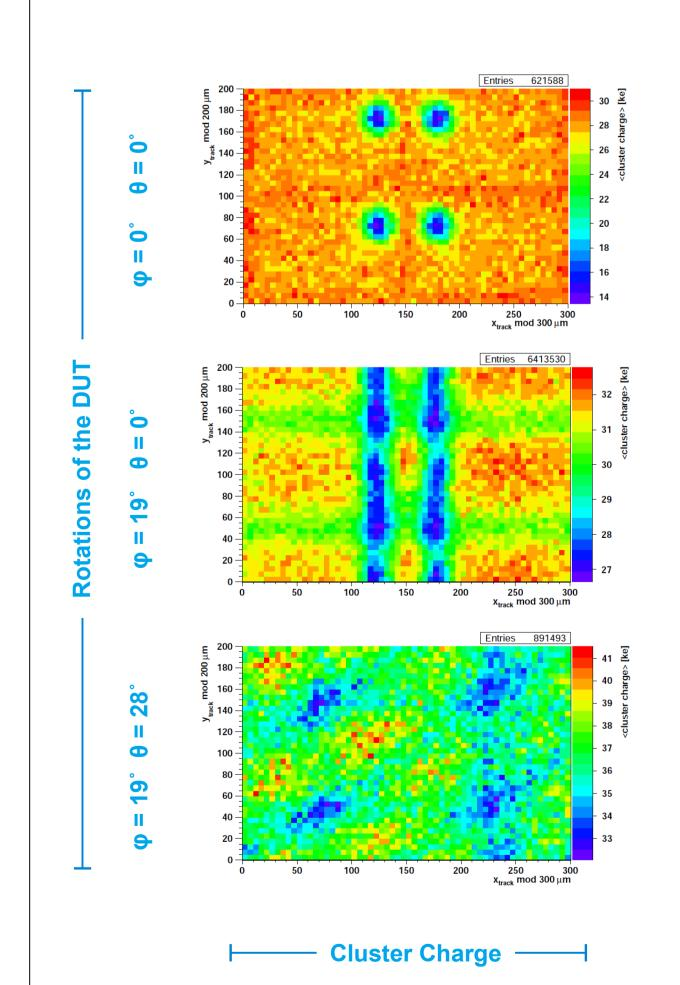
The high resolution of the beam telescope tracks have been used to study various effects within single pixel cells of the CMS Pixel sensor at different incidence angles. The maps show the four pixel cells of the sensor photograph at the head of the page. All matched tracks within the fiducial volume have been folded into these maps.
