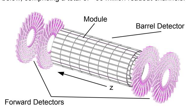
With the good performance of the LHC delivering two times the design luminosity an upgrade of the CMS Pixel Detector is required to maintain and extend the tracking efficiency.
