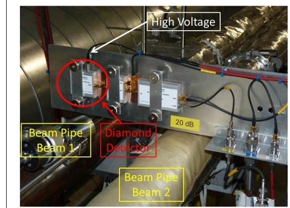
**Installation of Diamond Detectors** Installation of pcCVD diamond detector above the beam pipe for beam loss measurements.
