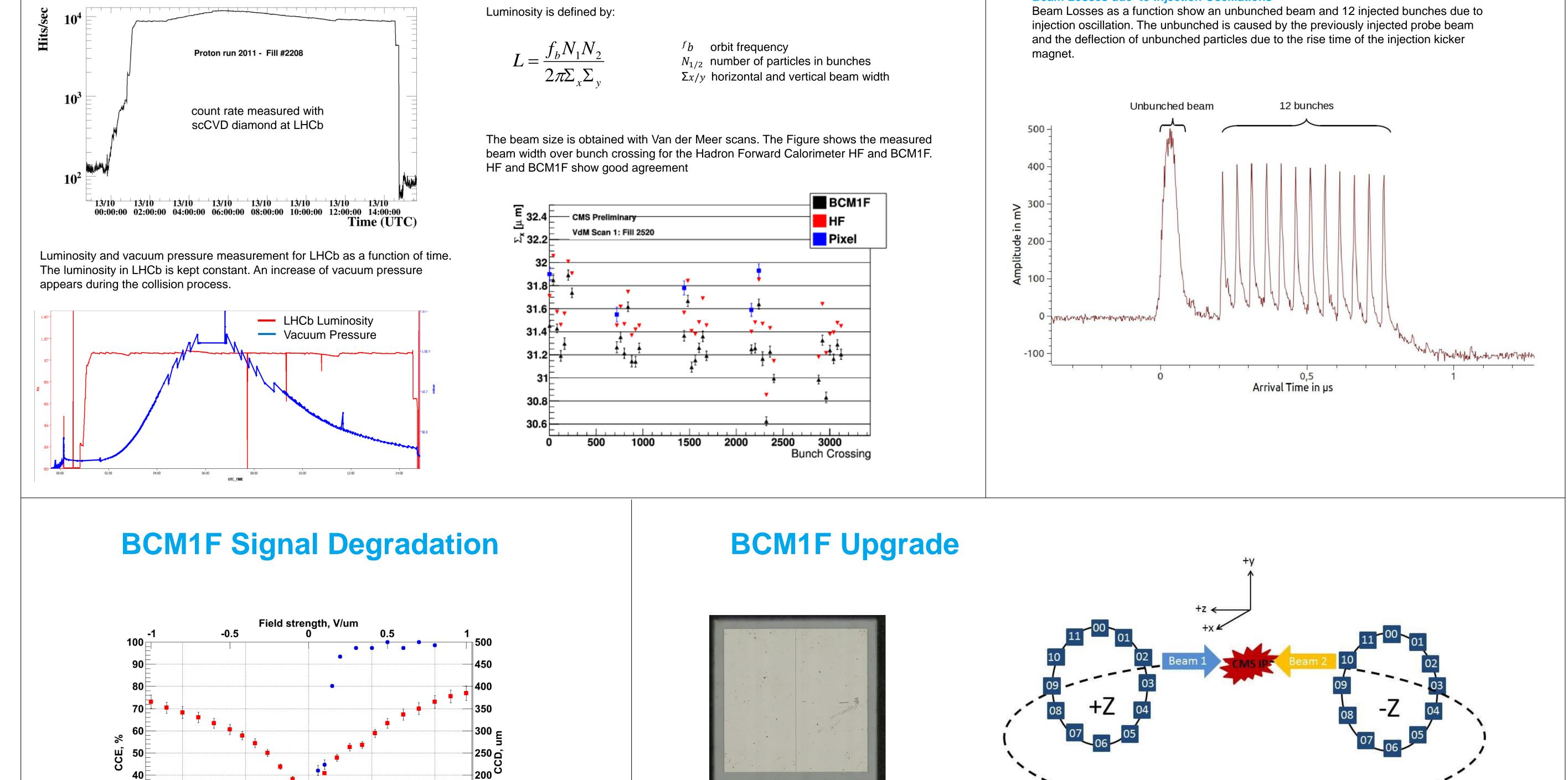
Luminosity Measurements with scCVD Sensors
