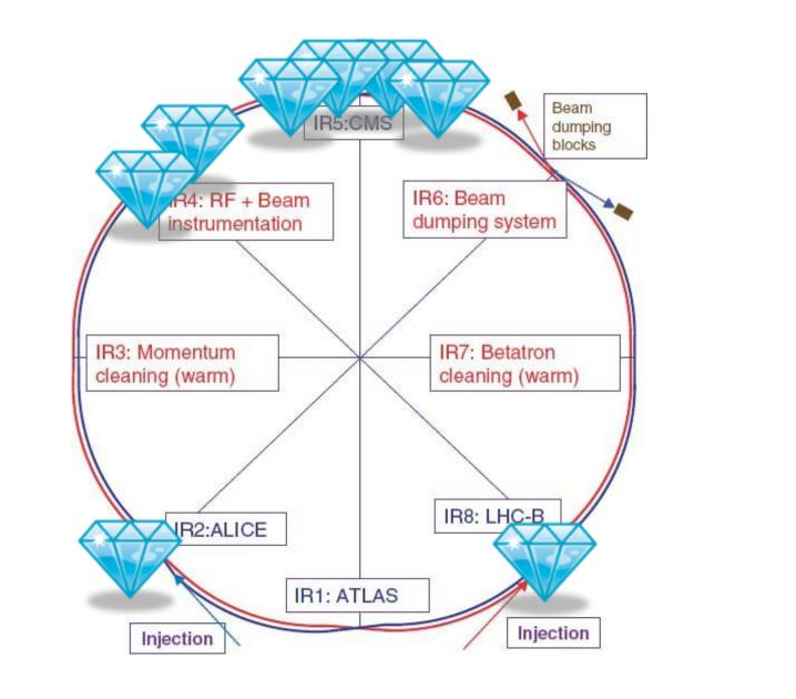
Diamond detectors based on scCVD diamond sensors are installed
